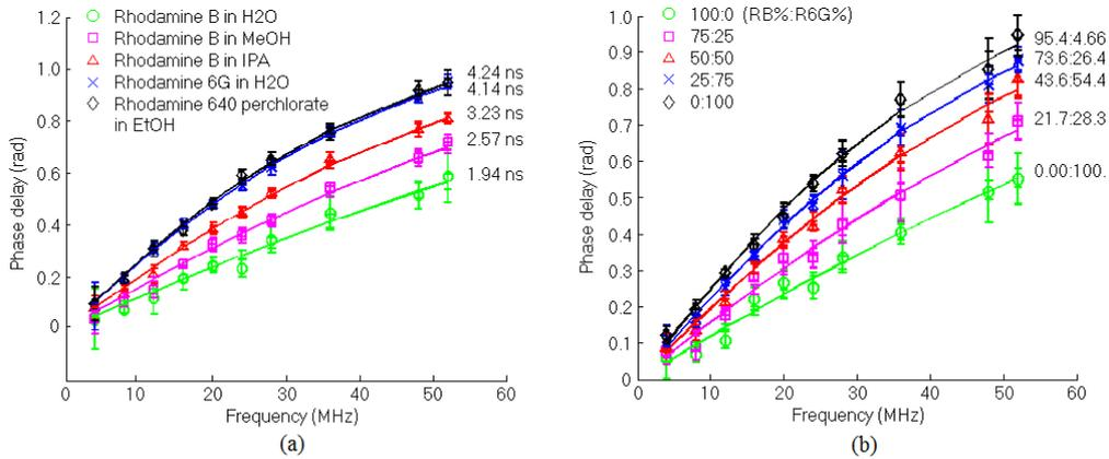
Fig. 3. (a) Selected fluorescence lifetime measurements. (b) Lifetime measurements of Rhodamine B / Rhodamine 6G mixtures at various ratios in water. The error bars denote the 95% confidence interval of the signal windows at each beat frequency. A non-linear fitting of Eq. (2) was applied to the data to extract the fluorescence lifetime values.
