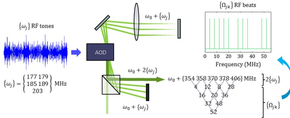
Fig. 2. Generation of multiple unique beat frequencies using the AOD and cat's-eye configuration. (a) Time domain signal of RF tones  $\{\omega_j\}$ . (b) The signal in (a) drives the AOD in the cat's-eye configuration to produce an optical beam containing frequency shifts of twice the input RF tone frequencies. (c) These RF tones are engineered to avoid beat frequency overlap, which causes phase ambiguity.
