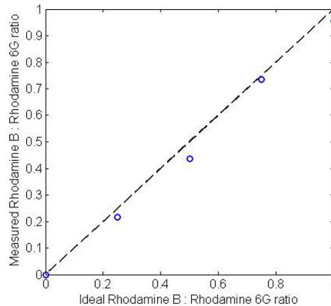
Fig. 4. Measured RB:R6G two-component mixtures at different component ratios (circles), as compared to the ideal case (dashed line).
