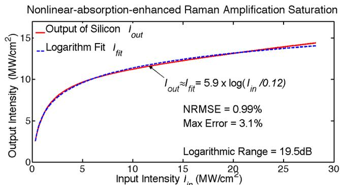
Fig. 1. Synthesis of the logarithmic computing primitive with the nonlinear-absorption-enhanced Raman amplification. The input Raman pump is 56.1 MW/cm<sup>2</sup> and the input non-degenerate TPA pump source is 50.1 MW/cm<sup>2</sup>. The output is fit to a logarithmic function over a 19.5 dB input range with a 0.99% normalized-mean-square error of 0.99% and a 3.1% maximum error.
