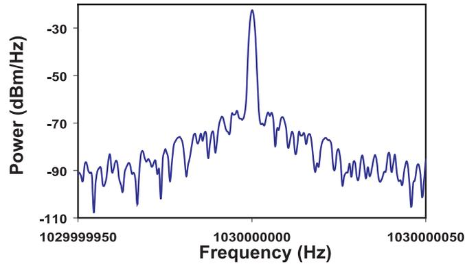
**Fig. 4.** Conversion of analog RF signal (centered at 1.03 GHz) from Stokes to anti-Stokes. Electrical SNR of 47 dBc was obtained over a bandwidth of 100 Hz.
