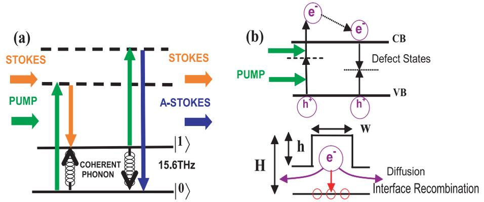
**Fig. 1.** (a) The vibrational energy levels of Silicon showing the Raman wavelength conversion process. (b) Electronic energy levels of Silicon and Two-photon absorption (TPA) process. Free carriers generated by TPA increase the overall loss. These free carriers diffuse out of the rib structure and also recombine at interface defect states. In this work,  $w = 2 \mu\text{m}$ ,  $H = 0.93 \mu\text{m}$  and  $h = 0.45 \mu\text{m}$ .
