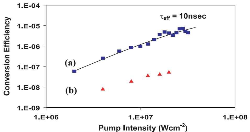
Fig. 3. Experimental plot of conversion efficiency vs. pump intensity: (a) both pump and signal are TE polarized (no birefringence). Theoretical fit shows good agreement for effective lifetimes  $\tau_{\text{eff}}$  of 10 nsec. (b) pump and signal are TE and TM polarized respectively (with birefringence).
