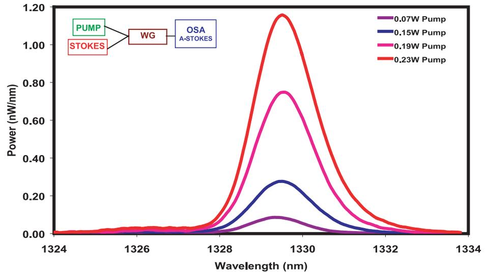
**Fig. 2.** The experimental setup used for wavelength conversion is shown in the inset. The pump signal (1427.3 nm) and Stokes signal (1542.3 nm) are launched into the waveguide. The propagation loss in these waveguides was  $\sim 2.5$  dB/cm. The converted anti-Stokes signal (1328.8 nm) is observed using the Optical spectrum analyzer (OSA). The optical spectrum of converted anti-Stokes signal is shown at various pump powers.
