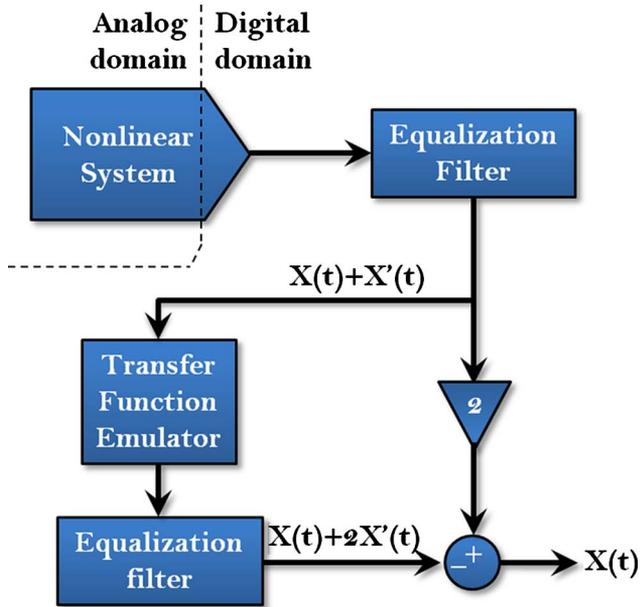
Fig. 1. (Color online) Block diagram of the demonstrated broadband linearization technique.
