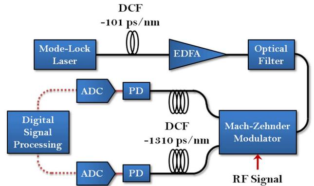
Fig. 2. (Color online) Experimental setup of the photonic TSADC to evaluate the broadband linearization technique. EDFA, Er-doped fiber amplifier; PD, photodetector; DCF, dispersion-compensating fiber; ADC, analog-to-digital converter.
