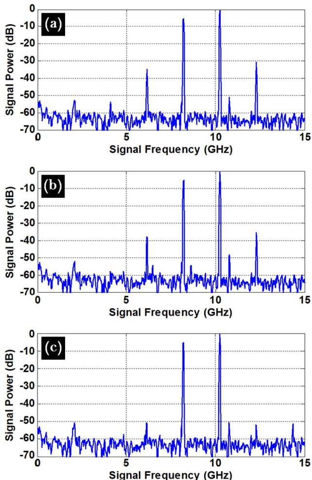
Fig. 3. (Color online) Signal power for a two-tone test ( $f_1 = 8.2$  GHz,  $f_2 = 10.25$  GHz) (a) before any corrections for nonlinearity, (b) after conventional arcsine operation, showing incomplete cancellation of intermodulation distortion, (c) after broadband linearization, showing drastic improvement of intermodulation distortions ( $2f_1 - f_2 = 6.15$  GHz and  $2f_2 - f_1 = 12.3$  GHz) over conventional arcsine operation.
