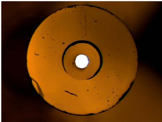
Fig. 1. (Color online) Optical micrograph of a cleaved cross section of the silica-clad germanium core optical fiber. Note the circularity and concentricity of the fiber and metallic appearance of the core. The crescent-shaped feature is a gap between concentric silica cladding tubes, used to achieve the desired core/clad ratio, that did not fully fuse together at the draw temperature.
