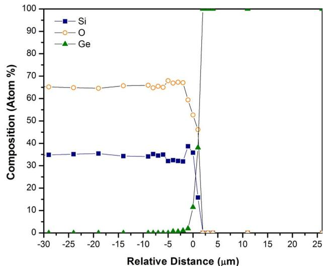
Fig. 2. (Color online) Elemental analysis of the silica-clad germanium core optical fiber. The cladding, negative relative distance, which represents the core/clad boundary, exhibits stoichiometric  $\text{SiO}_2$ . The core, positive relative distance, is found to be entirely germanium to within the tolerance of the measurement.
