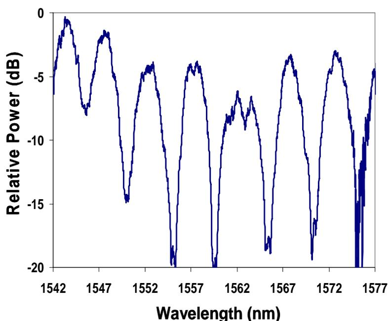
Fig. 6. Spectral characteristics of the thru port of the multistage microdisk filter device. Non-resonant wavelengths are collected at the thru port of the device. By comparing with Fig. 5, it may be seen that every peak in Fig. 5 corresponds to a dip in Fig. 6.
