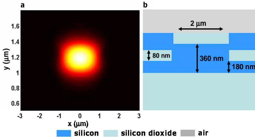
Fig. 3. The electric field profile of the fundamental mode of a waveguide in the second silicon layer. a) Fundamental mode field profile of the waveguides defined in the second silicon layer, calculated using a finite element mode solver. b) Waveguide structure used for the simulation results shown in part a, which closely matches the experimentally observed structure, with a discontinuous oxide layer, shown in Fig. 2.
