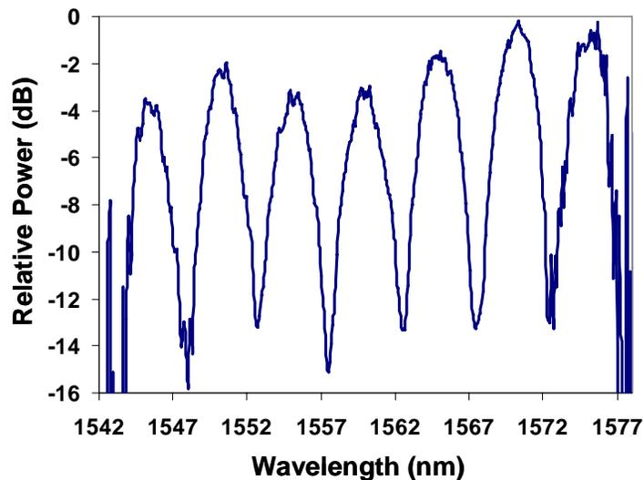
Fig. 5. Spectral characteristics of the drop port of the multistage microdisk filter device. Wavelengths that are resonant with the microdisk structure travel through the multilayer structure and get collected at the drop port of the device. Non-resonant wavelengths are collected at the thru port of the device.
