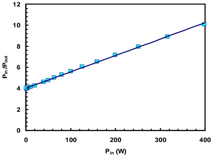
Fig. 6. TPA measurement result. The input power,  $P_{in}$ , is not corrected for coupling losses. The linear behavior is maintained up to  $\sim 400$  W.
