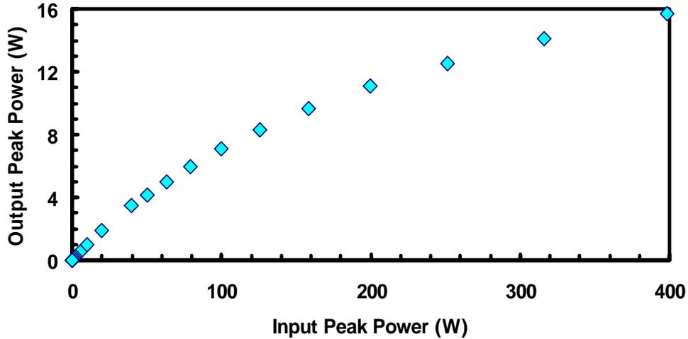
Fig. 5. Output power vs. input power results, using a mode-locked laser, and depicting a nonlinear relationship.
