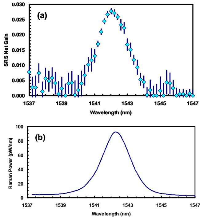
Fig. 2. (a) Measured spectral characteristic of the Stimulated Raman Scattering (SRS) in the silicon waveguide. The error bars are the standard deviation from this average. The pump power was 0.64 W at the front facet of the waveguide. SRS Net Gain is the ratio of the amplitude of the LIA output to the average signal power throughput. (b) Spontaneous Raman Spectra of the same waveguide with the same pump power as in (a).
