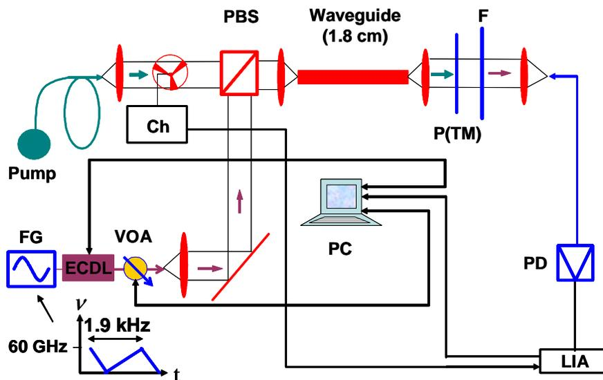
Fig. 1. Experimental setup: Pump-CRC fiber laser; Ch-Chopper; PBS-Polarization Beam Splitter; LIA- Lock-in amplifier; ECDL-External cavity diode laser (tunable); FG-Function generator (60 GHz freq. range); VOA-Variable optical attenuator; PD-optically-broadband photodetector. Thick lines represent electrical connections and wiring, thin lines represent free-space optical beams, and colored lines represent optical fiber.
