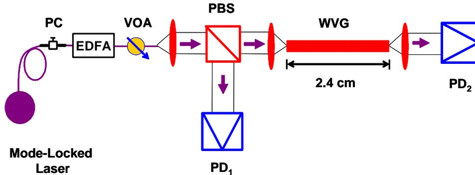
Fig. 4. Experimental setup for measuring TPA. The waveguide in this case is different from the one used for SRS. PC-Polarization controller; VOA-Variable optical attenuator; PBS – Polarization beam splitter; PD<sub>1</sub> and PD<sub>2</sub> photo-detectors (identical, Newport 1830-C).
