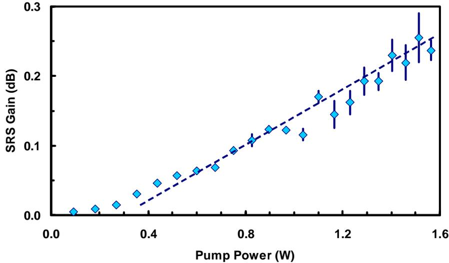
Fig. 3. The maxima from each spectral scan are plotted against effective pump power coupled into the front facet of the waveguide. A maximum of 0.25 dB (6%) amplification is obtained.
