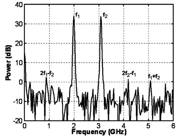
Fig. 6. Measured digital magnitude spectrum using two-tone test.
