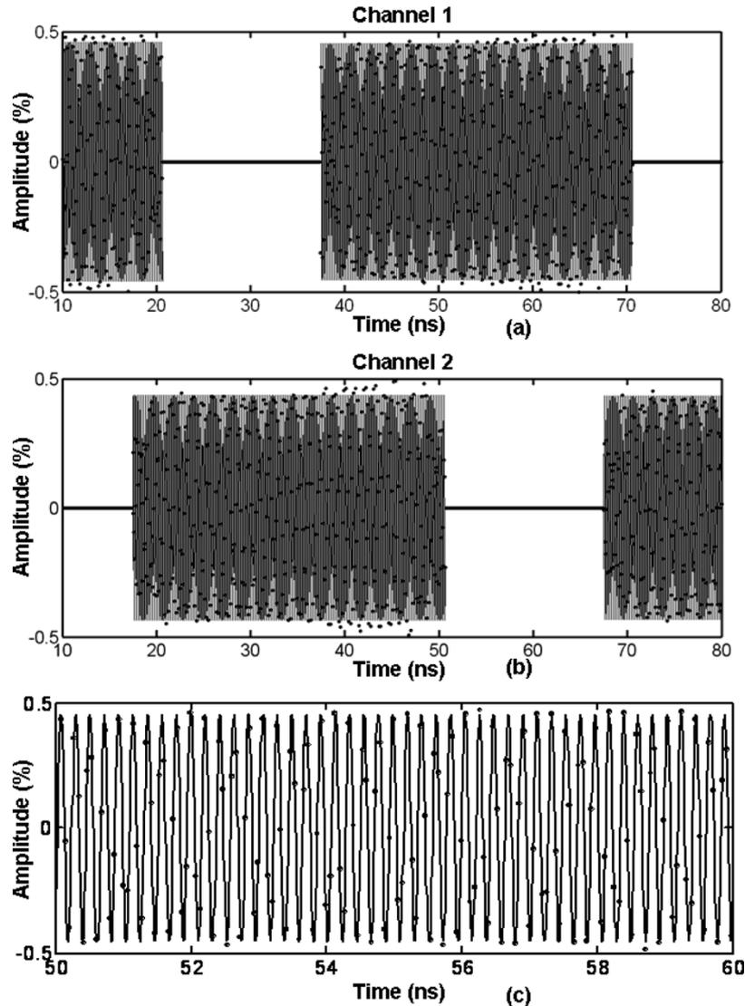
Fig. 7. Measured 4.7-GHz signal after interleaving. The symbols are sample points and the line is the fitted sine curve. (a) Channel 1 at 1576 nm. (b) Channel 2 at 1594 nm. (c) Portion of (a).
