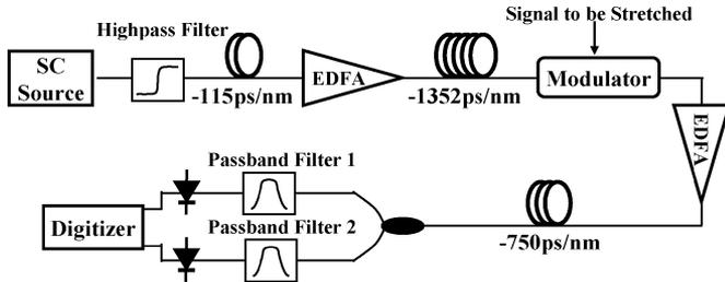
Fig. 4. Experiment setup for a two-channel continuous-time stretch ADC. SC: Supercontinuum. EDFA: Erbium-Doped Fiber Amplifier. Highpass filter: 1570 nm above. PB filter 1: 1576 nm with 20-nm bandwidth. PB filter 2: 1594 nm with 20-nm bandwidth.
