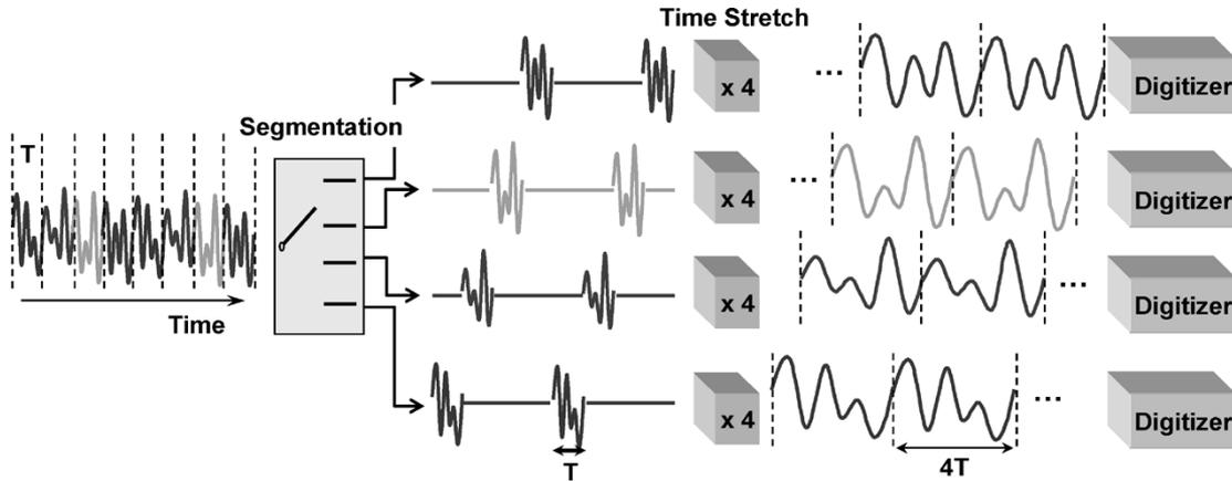
Fig. 2. Conceptual diagram of continuous-time stretched ADC.
