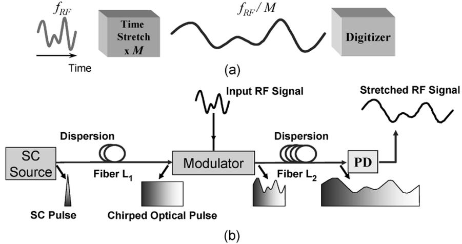
Fig. 1. (a) Conceptual block diagram of time-stretched ADC. (b) Schematic diagram of the photonic implementation of time stretch.
