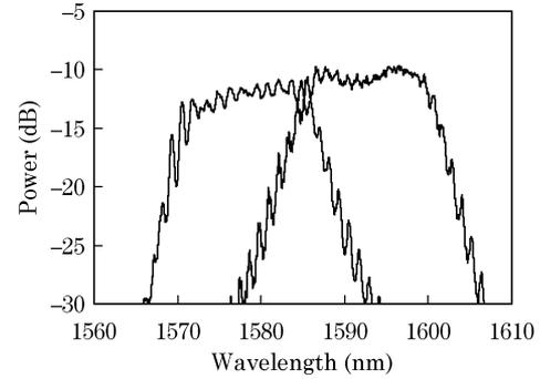
Fig. 5. Optical spectrum of two channels used in the continuous-time stretch experiment.
