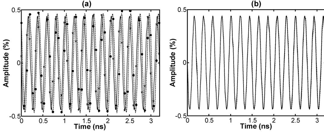
Fig. 8. Overlap between two adjacent channels. The star and circular symbols represent the sample points of two channels, respectively. The solid and dashed lines are the fitted curves. (a) Precalibration where gain and time mismatches are visible. (b) Postcalibration.
