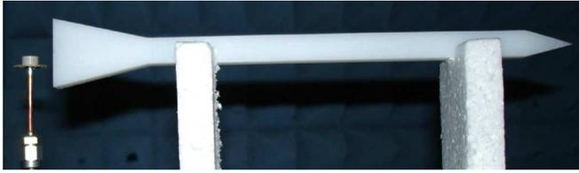
Fig. 5. Measurement setup of DFE coupling to the  $TM_{010+\delta}$  mode monopole DRA.
