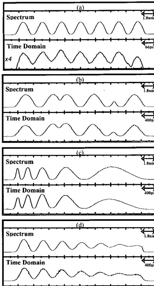
Figure 5. (a) 12.1 GHz Tone (b) PM (c) FM (d) AM modulations shown both in spectrum and time domains.
