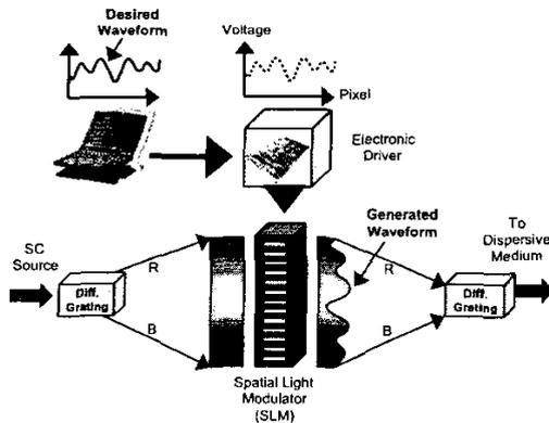
Figure 3. A desired waveform is sent to an electronic driver which determines the voltage for each liquid crystal pixel. The SLM performs spectral shaping to a dispersed broadband pulse.
