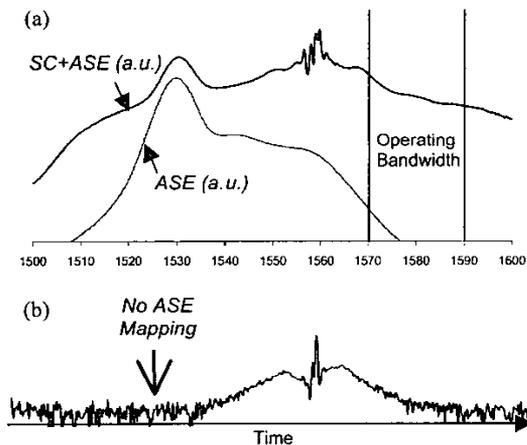
**Figure 7.** (a) The system is chosen to operate away from the ASE peak at 1530 nm to avoid distortion, (b) Time domain waveform showing the absence of wavelength-to-time mapping in the ASE dominated portion of the SC spectrum.
