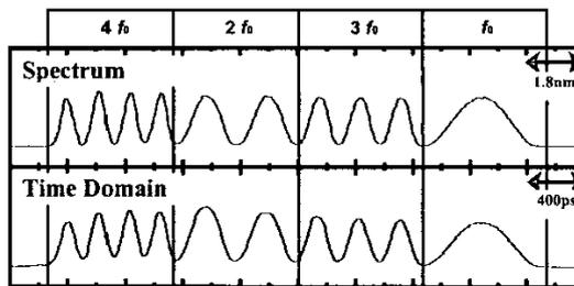
Figure 6. Ultra-wide-band Frequency Hopped CDMA. The frequency hops from 1.25 GHz to 5 GHz in increments of 1.25 GHz.
