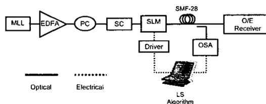
**Figure 1.** Block diagram of AWG. MLL: Mode Locked Laser. PC: Polarization Controller. SC: Supercontinuum. SLM: Spatial Light Modulator. OSA: Optical Spectrum Analyzer.
