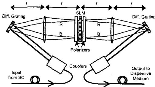
Figure 2. Experimental setup of SLM in a 4- $f$  grating and lens configuration [1].
