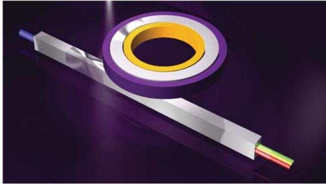
Fig. 12. Schematic of the integrated cascaded cavity Raman laser using a microresonator structure.
