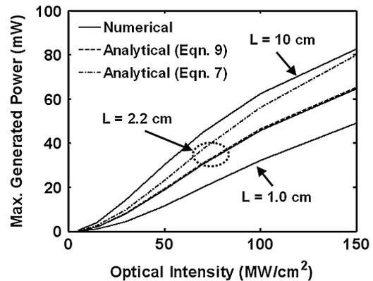
Fig. 5. Simulated maximum power generation (solid lines) versus coupled pump intensity for three different device lengths of 1.0, 2.2, and 10 cm. Also shown are the analytical values from the approximate form in (7) (dot-dashed line) and the exact expression in (9) (dashed line) for the 2.2-cm case.
