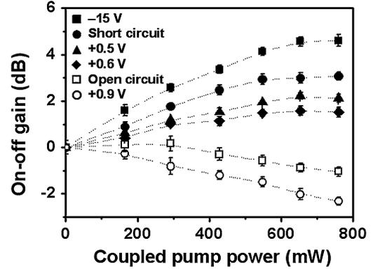
Fig. 2. Measured on–off Raman gain versus coupled pump power in the devices of Fig. 1 at different biasing conditions.
