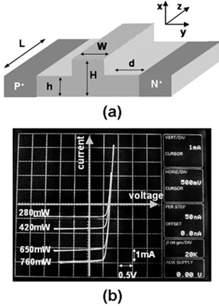
Fig. 1. (a) Schematic of a silicon waveguide with a p-n junction diode. The values of the shown geometrical dimensions are given in Table I. (b) Current-voltage characteristics of the fabricated p-n diodes measured with a curve tracer at various coupled pump powers, showing photovoltaic effect in the fourth quadrant (current < 0 and voltage > 0).
