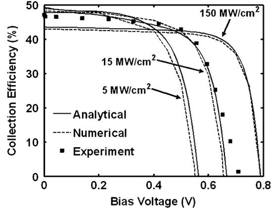
Fig. 4. Collection efficiency of the photovoltaic effect at three pump intensities for analytical expressions (solid line), numerical simulations (dashed line), and experiment (squares).
