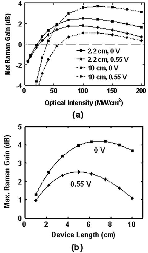
Fig. 7. (a) Simulated net Raman gain versus coupled pump intensity at short-circuit or 0 V (squares), and 0.55 V (diamonds) for devices with lengths of 2.2 cm (solid line) and 10 cm (dot-dashed line). (b) Maximum attainable net Raman gain versus device length for the same biases. Solid lines are fittings to the simulated data.
