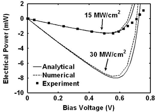
Fig. 3. Power–voltage characteristics of the diodes at two coupled pump intensities for analytical expressions (solid line), numerical simulations (dashed line), and experiment (squares).
