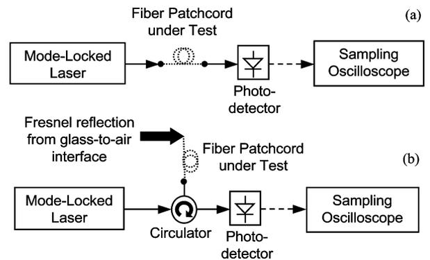
Fig. 5. Setup for accurately measuring group delay in a fiber patchcord connectorized on (a) both sides and (b) one side.
