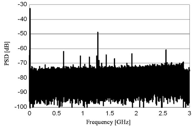
Fig. 9. Homodyne mixing spectral terms on the RF spectrum analyzer.
