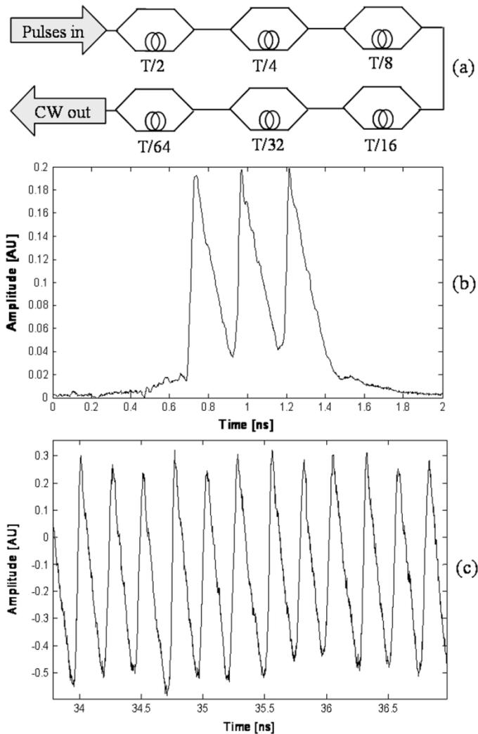
Fig. 4. Creation of a continuous waveform from modulated pulses. (a) Six-stage pulse repetition rate multiplier. (b) Three sawtooth periods produced by the PAWG. (c) Continuous 3.84-GHz sawtooth after the repetition rate multiplier.
