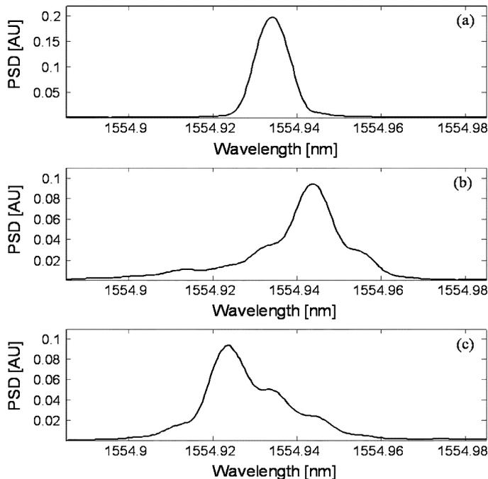
Fig. 8. Results of serrodyne frequency shifting observed on the OSA. (a) Initial, (b) downshifted, and (c) upshifted spectra are shown.
