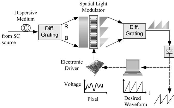
Fig. 2. Conceptual diagram of the RF photonic AWG. Note that the voltage applied to the SLM differs from the desired waveform to compensate for the system distortions.
