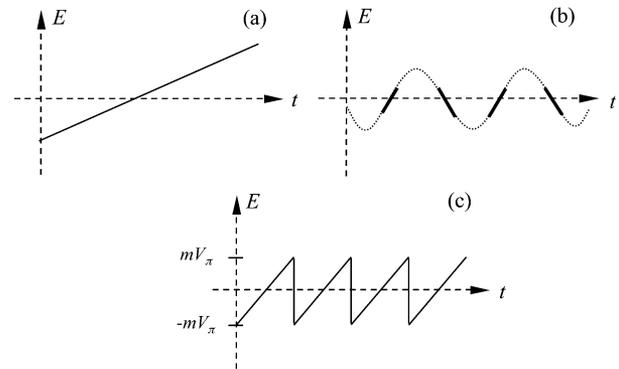
Fig. 1. Electric field temporal profiles that can be used for electrooptic frequency shifting. (a) Linear electric field. (b) Linear parts of a sinusoid. (c) Sawtooth with amplitude  $2mV_\pi$ .
