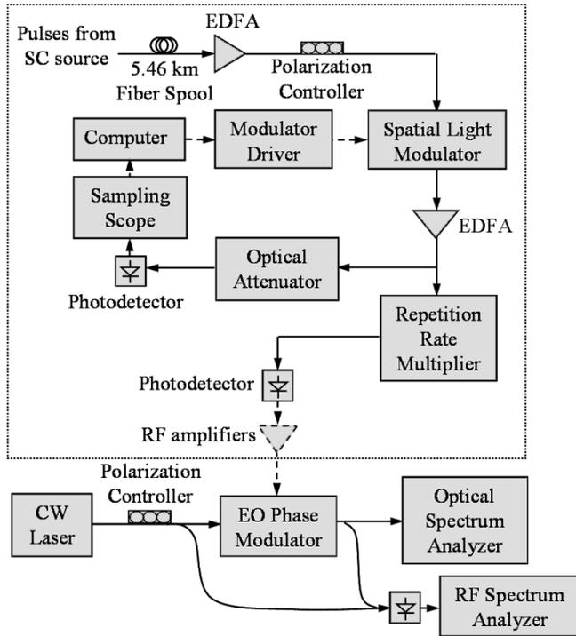
Fig. 7. Block diagram of the serrodyne frequency translator. Solid lines represent optical signals, dashed lines represent electrical signals, and the dotted line encloses the PAWG used to generate the sawtooth.
