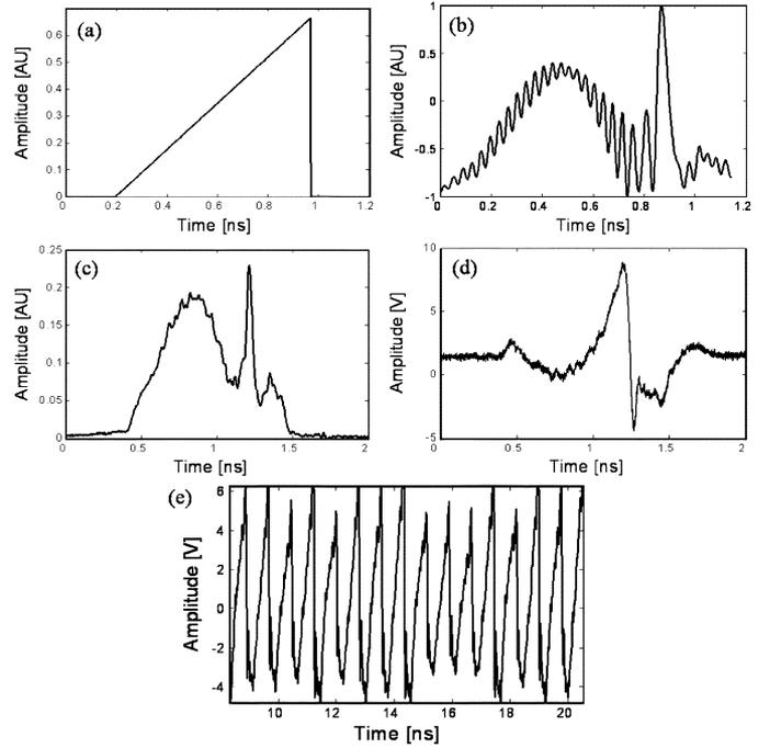
Fig. 6. High power sawtooth produced using the predistortion technique. (a) Desired sawtooth ramp. (b) Calculated predistorted ramp. (c) Predistorted ramp produced by SLM. (d) Amplified predistorted ramp. (e) Continuous sawtooth.
