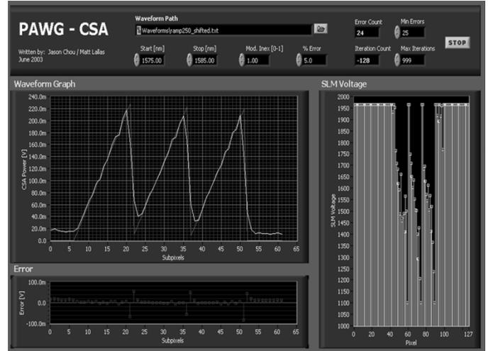
Fig. 3. PAWG LabVIEW user interface showing (top left) the desired and actual waveforms, (bottom left) the difference between them for each SLM pixel, and (right) the voltage applied to each SLM pixel.
