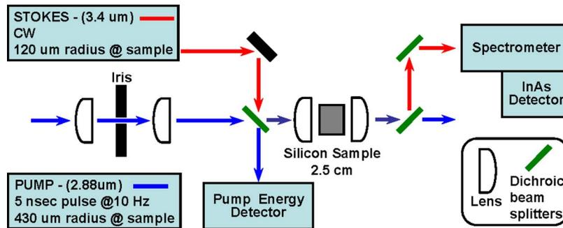
Fig. 1. The experimental setup.
