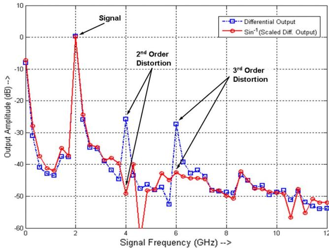
Fig. 5. Amplitude as a function of frequency for a 2-GHz input tone in a TS-ADC showing that the arcsine operation suppresses the second harmonic due to the Mach–Zehnder bias error and the third harmonic due to its transfer function. Note that the frequency scale corresponds to the original (prestretch) RF-signal frequency.
