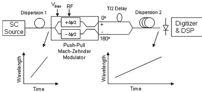
Fig. 3. TS-ADC with differential operation (SC = supercontinuum source).
