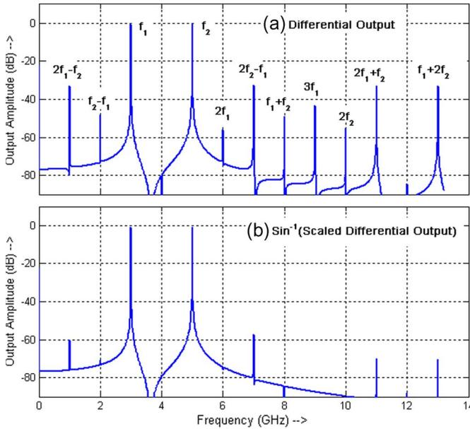
Fig. 2. Spectra for a two-tone test for an analog optical link with 3- and 5-GHz RF input frequencies. (a) Output amplitude as a function of frequency showing second- and third-order distortion tones caused by the Mach-Zehnder bias error and transfer characteristics. (b) Output spectrum with the distortions suppressed by the arcsine operation.
