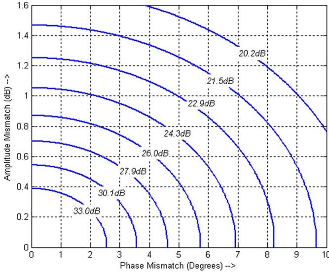
Fig. 7. Contour plots for DRRs that can be achieved as a function of amplitude and phase mismatches between the two differential channels.
