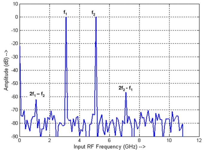
Fig. 6. Amplitude as a function of frequency calculated for a two-tone input with a 10-b electronic quantizer in a differential TS-ADC. Note that the frequency scale corresponds to the original (prestretch) RF-signal frequency.
