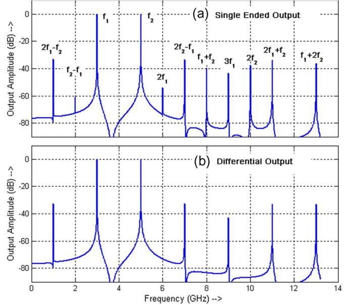
Fig. 1. Spectra of a two-tone test for an analog optical link with 3- and 5-GHz input frequencies and perfect Mach–Zehnder bias. (a) Single-ended output showing both second- and third-order distortion tones. (b) Output using differential operation showing that the dispersion-induced second-order distortion tones are rejected.
