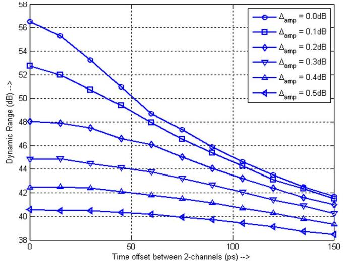
Fig. 8. Calculations of the dynamic range of the TS-ADC as a function of timing offsets between the two channels for different amplitude mismatch values.
