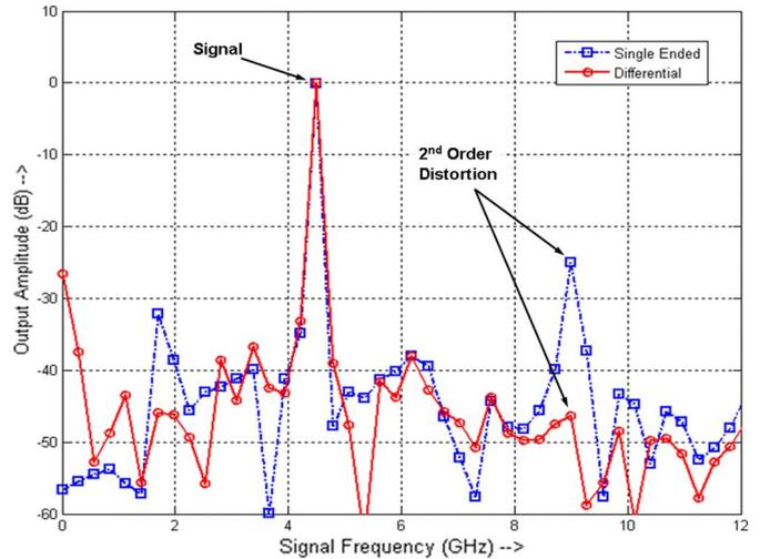
Fig. 4. Amplitude as a function of frequency for a 4.5-GHz RF input tone. The second harmonic at 9 GHz is suppressed by the differential operation. Note that the frequency scale corresponds to the original (prestretch) RF-signal frequency.
