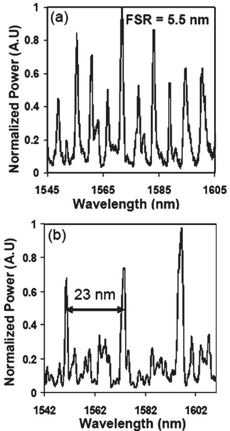
Fig. 18. Drop-port characteristics of (a) device consisting of cascaded microdisks with identical radii [20  $\mu\text{m}$ ] and (b) vernier filters made using microdisks of radii 20 and 25  $\mu\text{m}$ .
