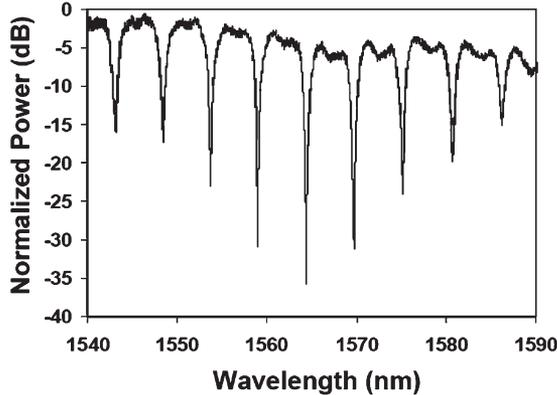
Fig. 6. Throughput port transmission characteristics of the microdisk resonator.
