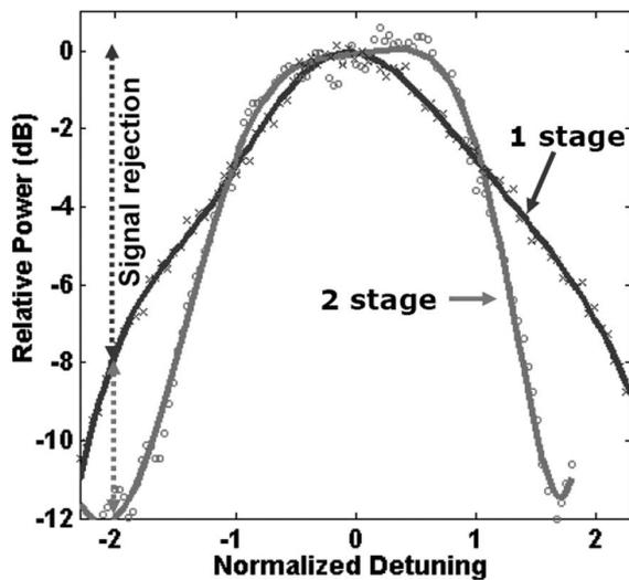
Fig. 13. Comparison of the filter characteristics of the two-stage device with a single-stage device, with frequency scale normalized to 3-dB bandwidths.
