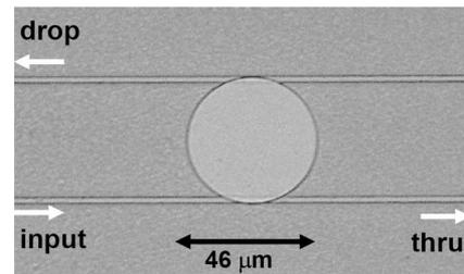
Fig. 4. Top view of a microdisk resonator vertically coupled to bus waveguides.
