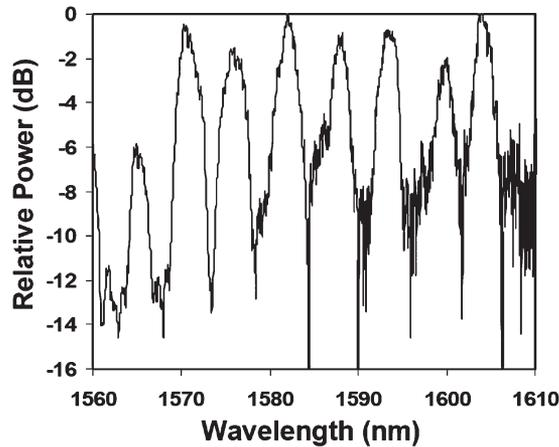
Fig. 12. Drop-port resonance characteristics of the cascaded device.
