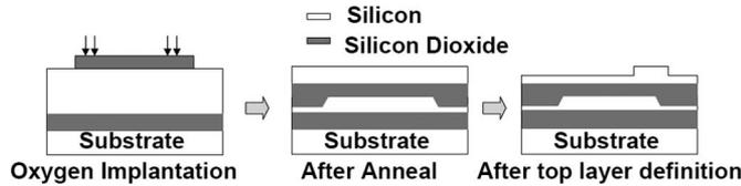
Fig. 1. Process flow of a SIMOX 3-D sculpting.
