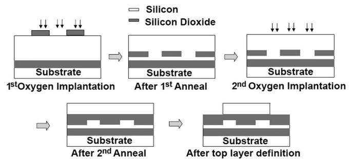
Fig. 15. Process flow of the modified SIMOX 3-D sculpting process for the fabrication of vernier filters.
