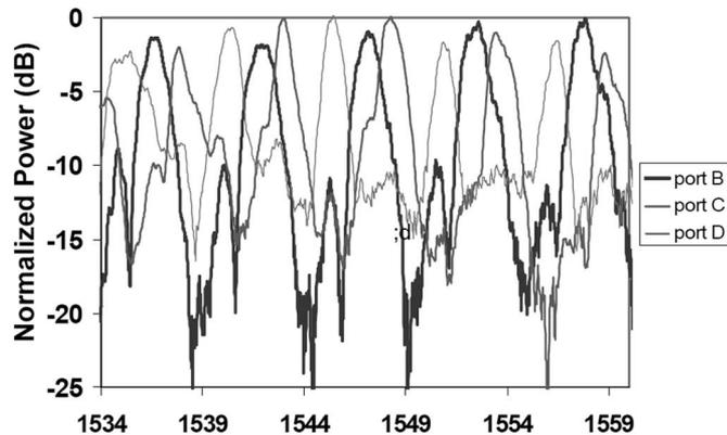
Fig. 9. Drop-port optical spectra of the 1 × 3 add-drop filter.
