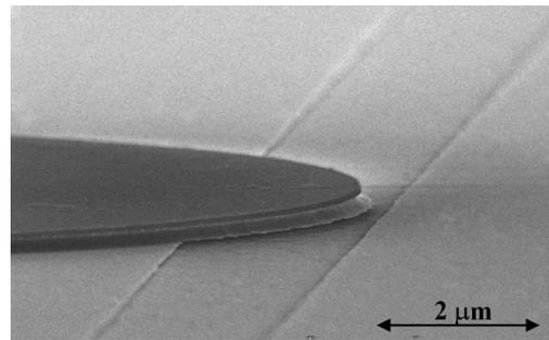
Fig. 3. SEM picture of the fabricated microdisk resonators of radius  $23 \mu\text{m}$  on the top silicon layer with bus waveguides underneath.
