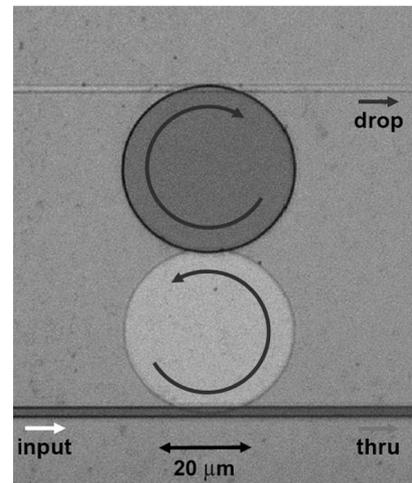
Fig. 11. Top view of the vertically coupled cascaded microdisk resonators.
