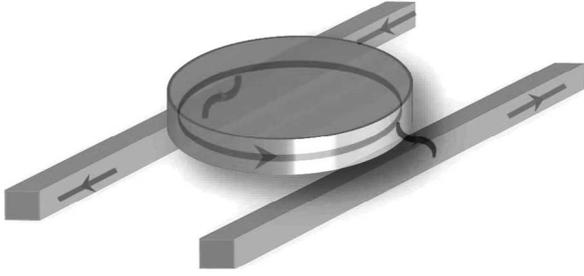
Fig. 19. Three-dimensional schematic of a microdisk resonators vertically coupled to bus waveguides illustrating the flow of optical energy.
