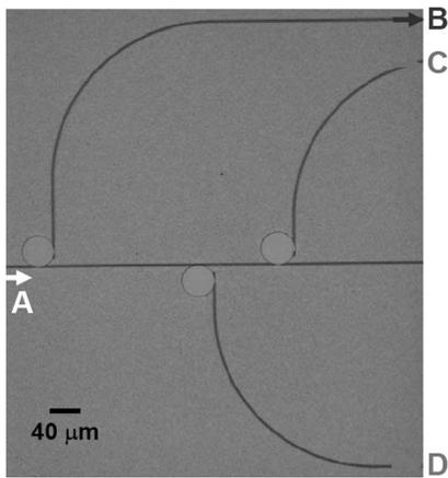
Fig. 8. Top view of the fabricated 1 × 3 add-drop multiplexer using disks of radii 20, 20.5, and 21 μm.
