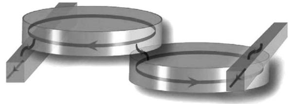
Fig. 10. Three-dimensional schematic of vertically coupled microdisk resonators and bus waveguides illustrating the flow of an optical energy.
