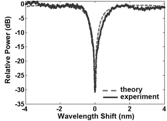
Fig. 7. Comparison of the experimental data with theory for the microdisk resonance at 1564.3 nm.
