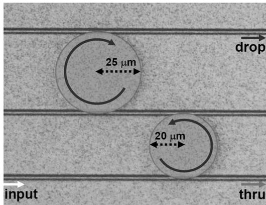
Fig. 17. Vernier filters made using microresonators of radii 20 and 25  $\mu\text{m}$ .
