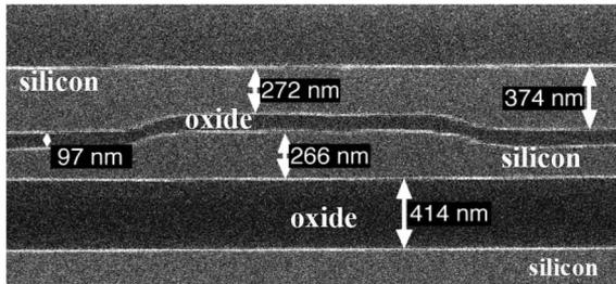
Fig. 2. Cross-sectional SEM view of the buried rib waveguide formed by the process of a SIMOX 3-D sculpting.
