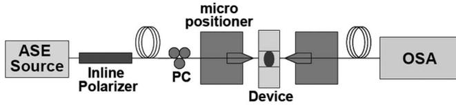
Fig. 5. Experimental setup used to characterize the microdisk resonators.
