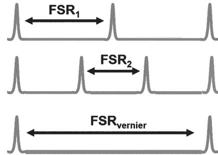
Fig. 14. Schematic depiction of the increase in FSR of a filter using vernier architecture.
