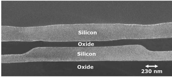
Fig. 16. Cross-sectional SEM view of the buried rib waveguide formed by a SIMOX 3-D sculpting employing two implantation steps.
