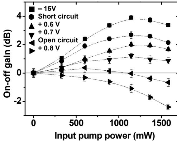
Fig. 2: Measured on-off Raman gain versus pump power in the devices of Fig. 1 at different biasing conditions.
