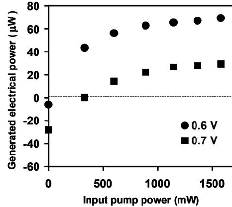
Fig. 3: Generated electrical power at different pump powers for two biases in the fourth quadrant.
