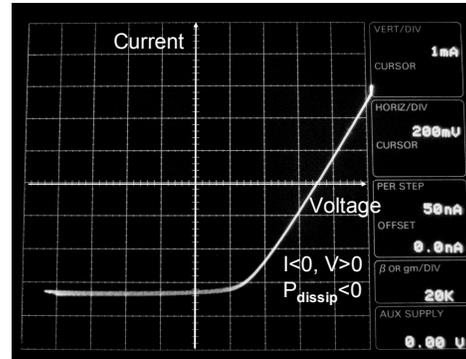
Fig. 4: The current-voltage characteristics of the p-n junction measured with a curve-tracer for an optical illumination of  $\sim 1.1$  W.
