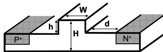
Fig. 1: Schematic of the silicon-on-insulator electrooptic modulator with a straddling p-n junction.
