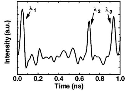
Fig. 3. Time-stretched spectral-coded output of encoder.  $\lambda_1 = 1554$  nm,  $\lambda_2 = 1554.8$  nm,  $\lambda_3 = 1555.6$  nm.
