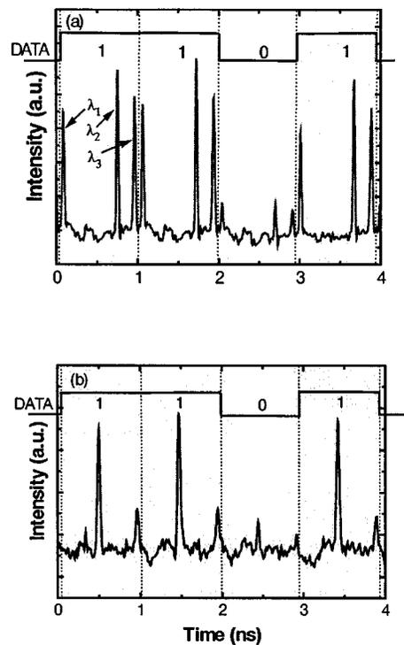
Fig. 5. (a) Encoded digital data at 1 Gb/s transmitted over 15-km DSF link. (b) Recovered data after matched decoder.
