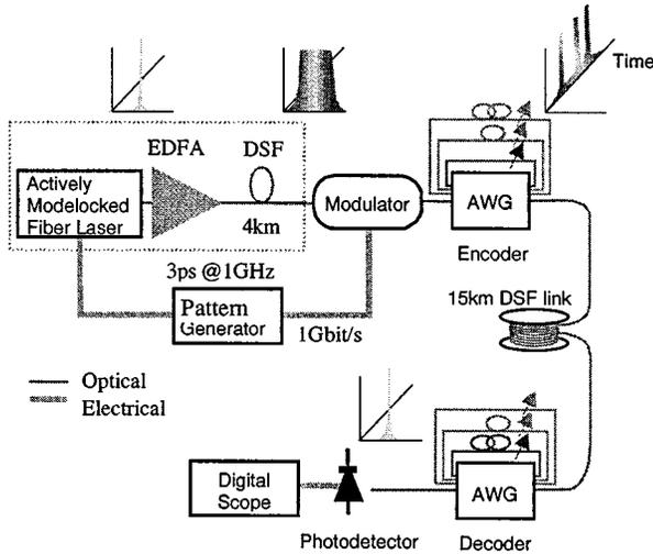
Fig. 1. Experimental setup of the wavelength-hopped time-spread OCDM system.
