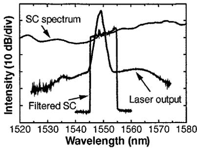
Fig. 2. Spectrum at the output of modelocked laser and after supercontinuum generation.
