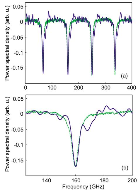
FIG. 6. (Color online) (a) Reconstructed gas spectrum from near-field measurements with  $D_1 \sim -695$  ps/nm,  $D_2 \sim -800$  ps/nm and 20 iterations with the temporal GS algorithm (blue trace). Spectrum recorded with optical spectrometer also shown (green trace, dashed). (b) Closeup view of a reconstructed line. Arbitrary frequency axis offset.
