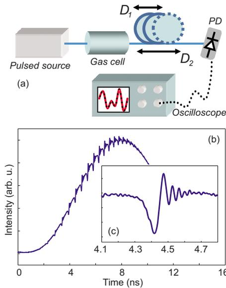
FIG. 5. (Color online) (a) Experimental setup for near-field measurements:  $D_1 \sim -695$  ps/nm,  $D_2 \sim -800$  ps/nm. (b) Pulse with encoded absorption lines measured with near-field dispersion  $D_1$ . (c) Closeup view of a near-field absorption line.
