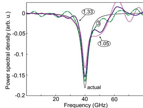
FIG. 4. (Color online) Recovered spectrum of a 5 GHz line after 20 iterations with  $D_1 = -600$  ps/nm and  $D_2/D_1 = 1.05$  (purple),  $D_2/D_1 = 1.33$  (blue), and  $D_2/D_1 = 3$  (green). Arbitrary frequency axis offset.
