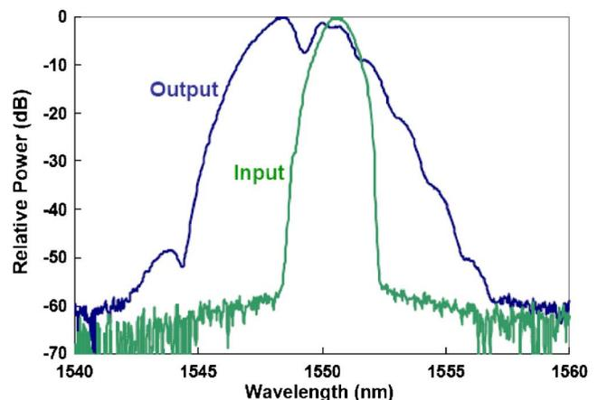
FIG. 4. (Color online) Spectral characteristics of the continuum generated in a silicon waveguide, along with the input spectrum.
