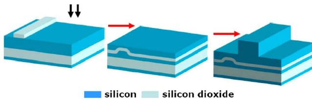
FIG. 2. (Color online) Schematic of the fabrication of three-dimensionally integrated structures using the process of SIMOX 3D sculpting.
