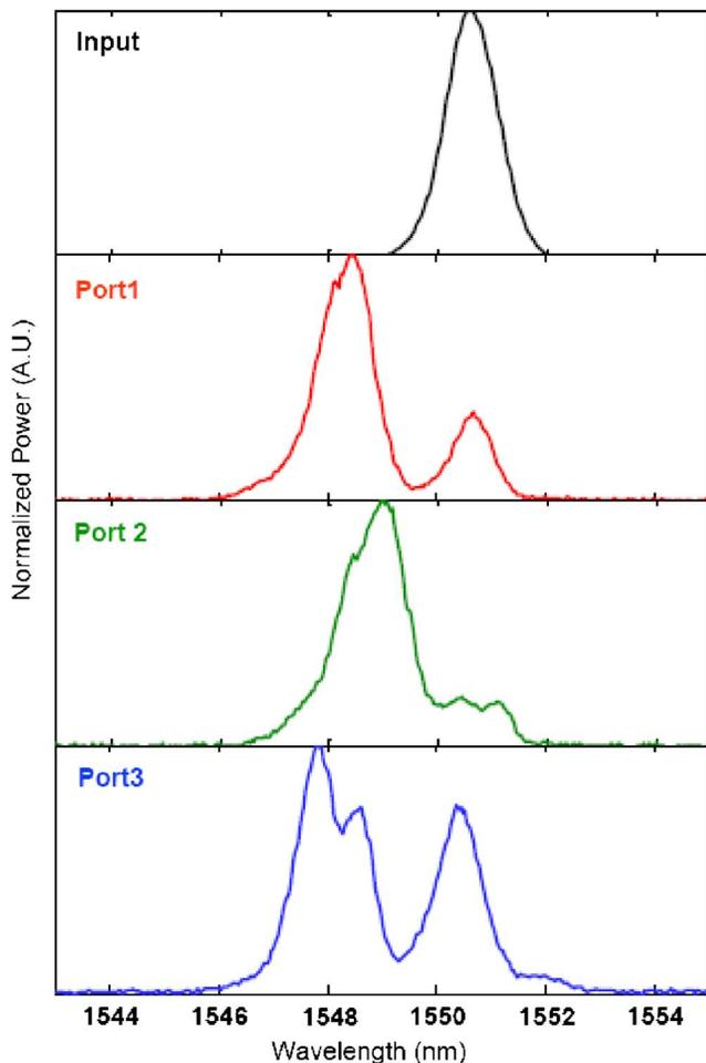
FIG. 5. (Color online) Wavelength channels generated by carving the continuum using microdisk resonators.
