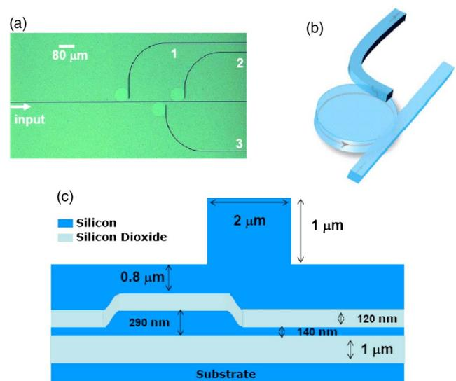
FIG. 3. (Color online) (a) Optical micrograph of the topview of the continuum carving device. (b) Magnified schematic of the coupling of the straight waveguide on the surface silicon layer to the microdisk resonator in the subsurface layer. (c) A cross sectional schematic of the device indicating the vertical dimensions of different layers and the width of the surface waveguide.
