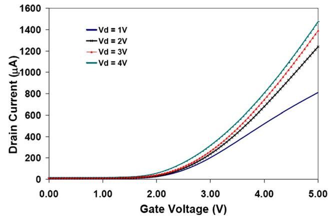
FIG. 3. Gate control characteristics ( $I_D$  vs  $V_G$ ) of the fabricated MOSFET.
