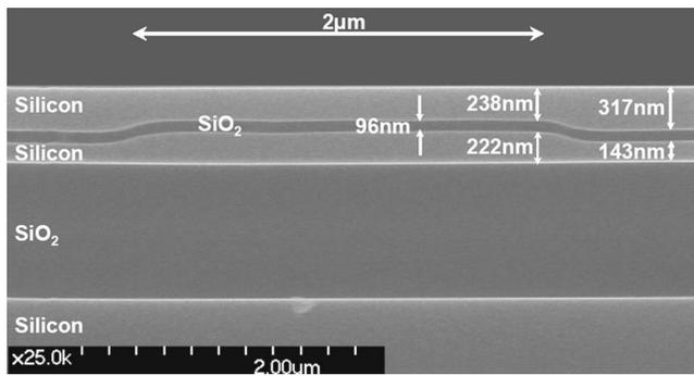
FIG. 1. Cross-sectional SEM of rib waveguides realized in the buried silicon layer. These waveguides act as bus waveguides to the microdisk resonator.
