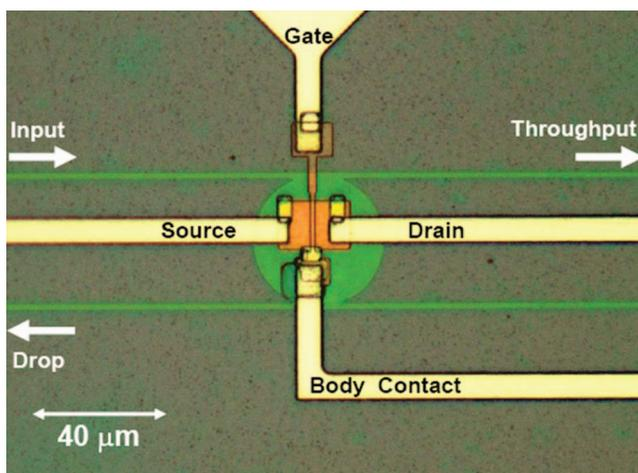
FIG. 2. (Color) Optical micrograph of a MOS transistor fabricated on the surface silicon layer, on top of a microdisk resonator that is situated in the buried silicon layer.
