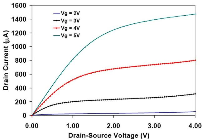
FIG. 4. Drain characteristics ( $I_D$  vs  $V_D$ ) of the fabricated MOSFET.
