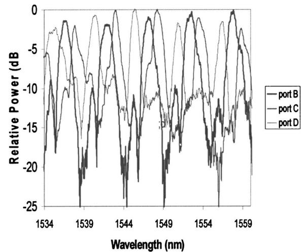
FIG. 6. Filter characteristics of the fabricated add-drop filter.
