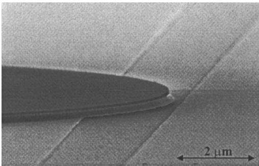
FIG. 3. SEM picture of the fabricated microdisk resonators on the top silicon layer with bus waveguides underneath.
