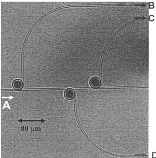
FIG. 4. Top view of the fabricated  $1 \times 3$  add-drop filter.
