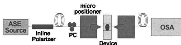
FIG. 5. Experimental setup used to characterize the add-drop filter.
