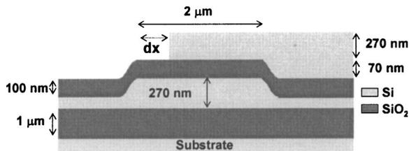
FIG. 2. Cross-sectional schematic depicting the coupling region between a buried waveguide and a microdisk resonator.
