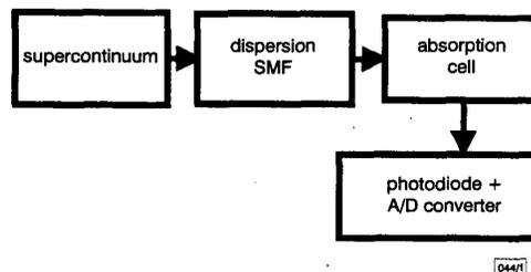
Fig. 1 Schematic diagram of time-domain spectrum characterisation
