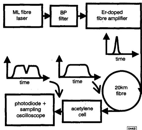
Fig. 2 Experimental setup for time-domain spectrum characterisation
