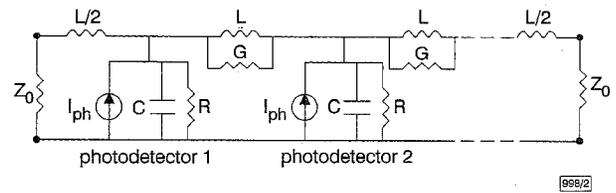
Fig. 2 Simple equivalent circuit for array described in text
